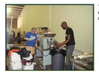
The bars are then poured into the hopper of an extruder where they are converted into small chips called "spiders."
